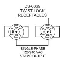
Figure 10. 120/240V Twist-Lock Auxiliary Receptacles
